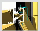
Concealed drainage holes are designed to shed water more efficiently.
